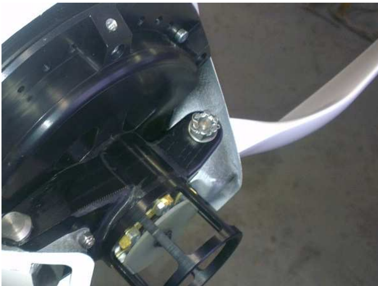
Fig.1 Propeller blades mounting on the holder
